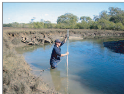
Collecting benthic invertebrates with a coring device.
